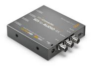
Mini Converter SDI to Audio 4K includes everything you need to de-embed 4 channels of analog audio or 8 channels of AES/EBU digital audio from any SDI video connection. Now you can access the audio in any SDI video connection for output to a massive range of audio equipment such as audio mixers, analog broadcast decks, audio monitors and more!
