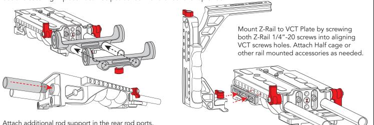
Attach additional rod support in the rear rod ports, by screwing in male threaded rods.
